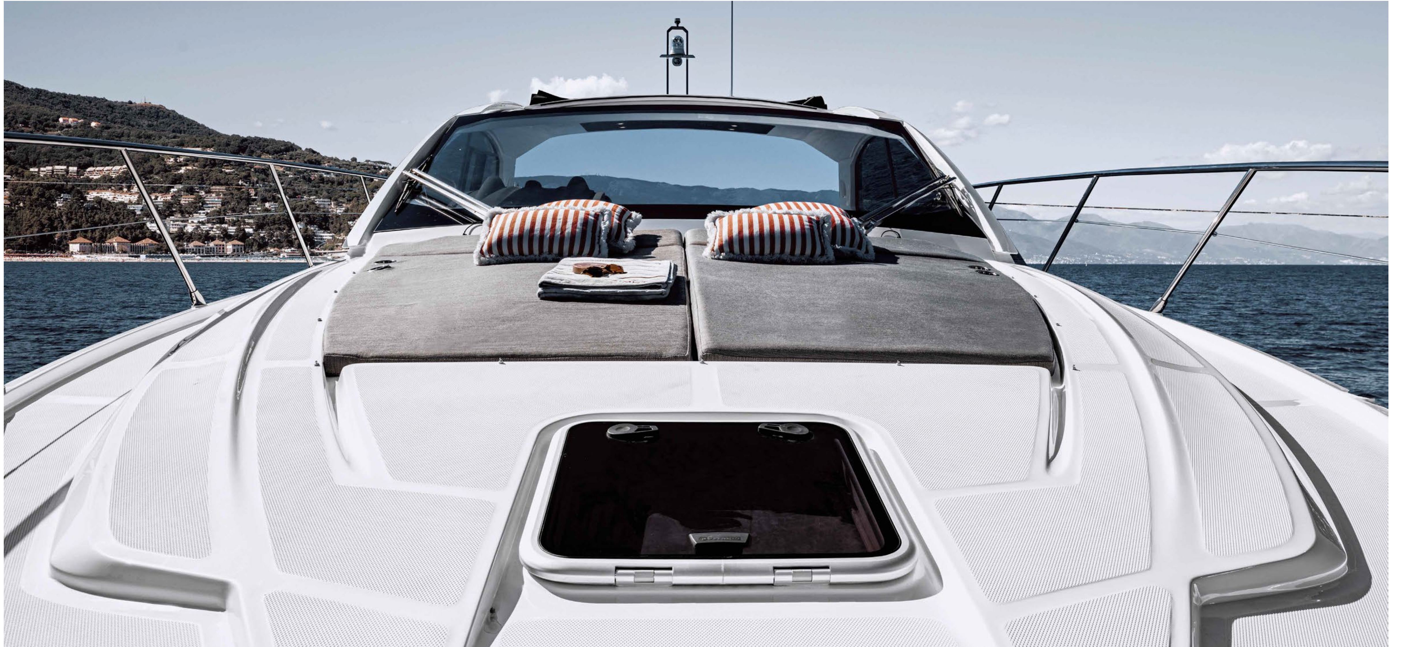
[ The unusual size of the single-piece curved windscreen improves visibility, interior perception of space and exterior aesthetics. Interior windows pillars are minimized to extend the effect. ]
