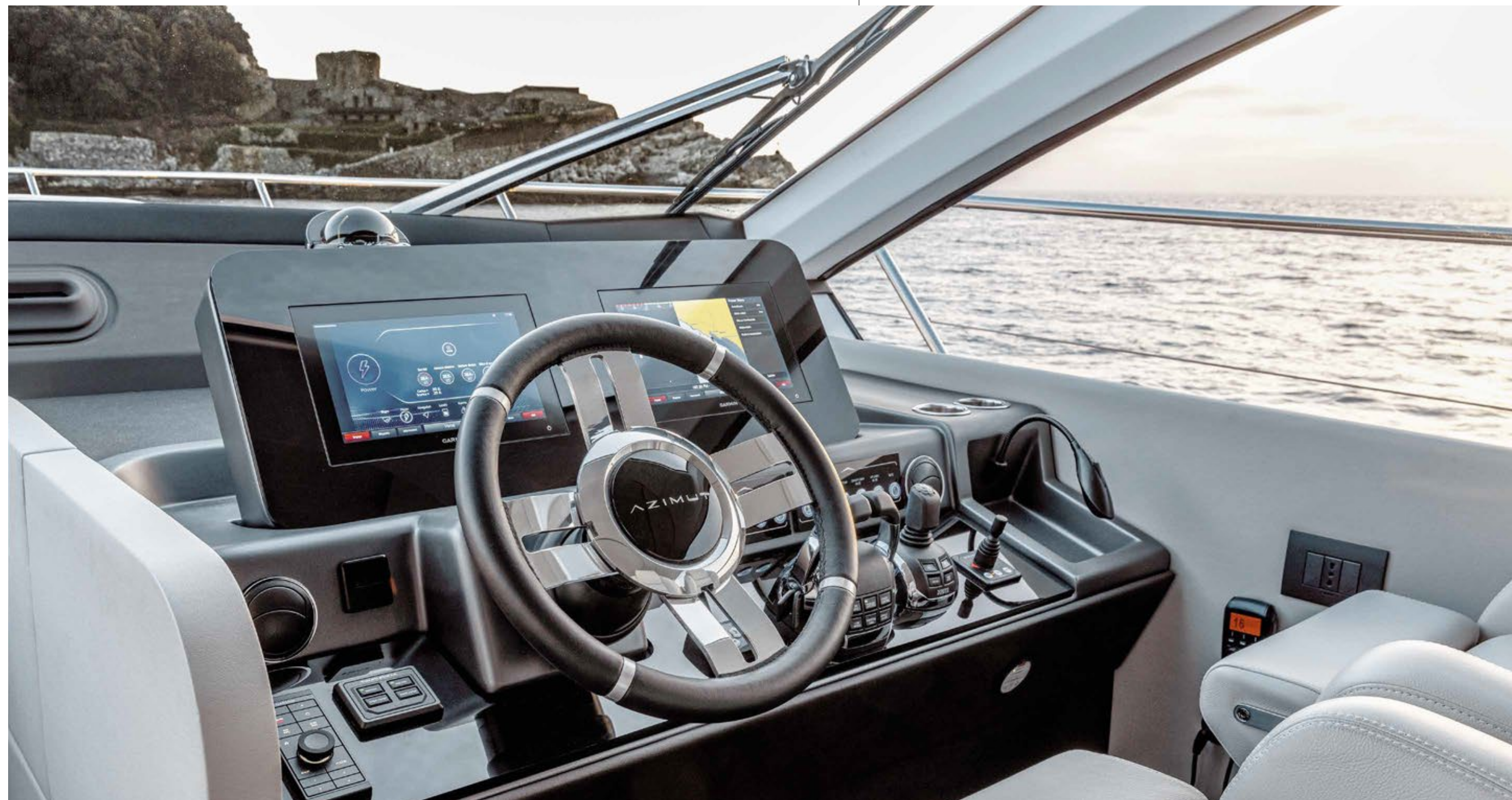
[ The control and monitoring system by Garmin has been customized to integrate the engines, alarms and tanks into their suite of helpful tools. The system can be accessed from both helm stations and remotely from a tablet. ]
