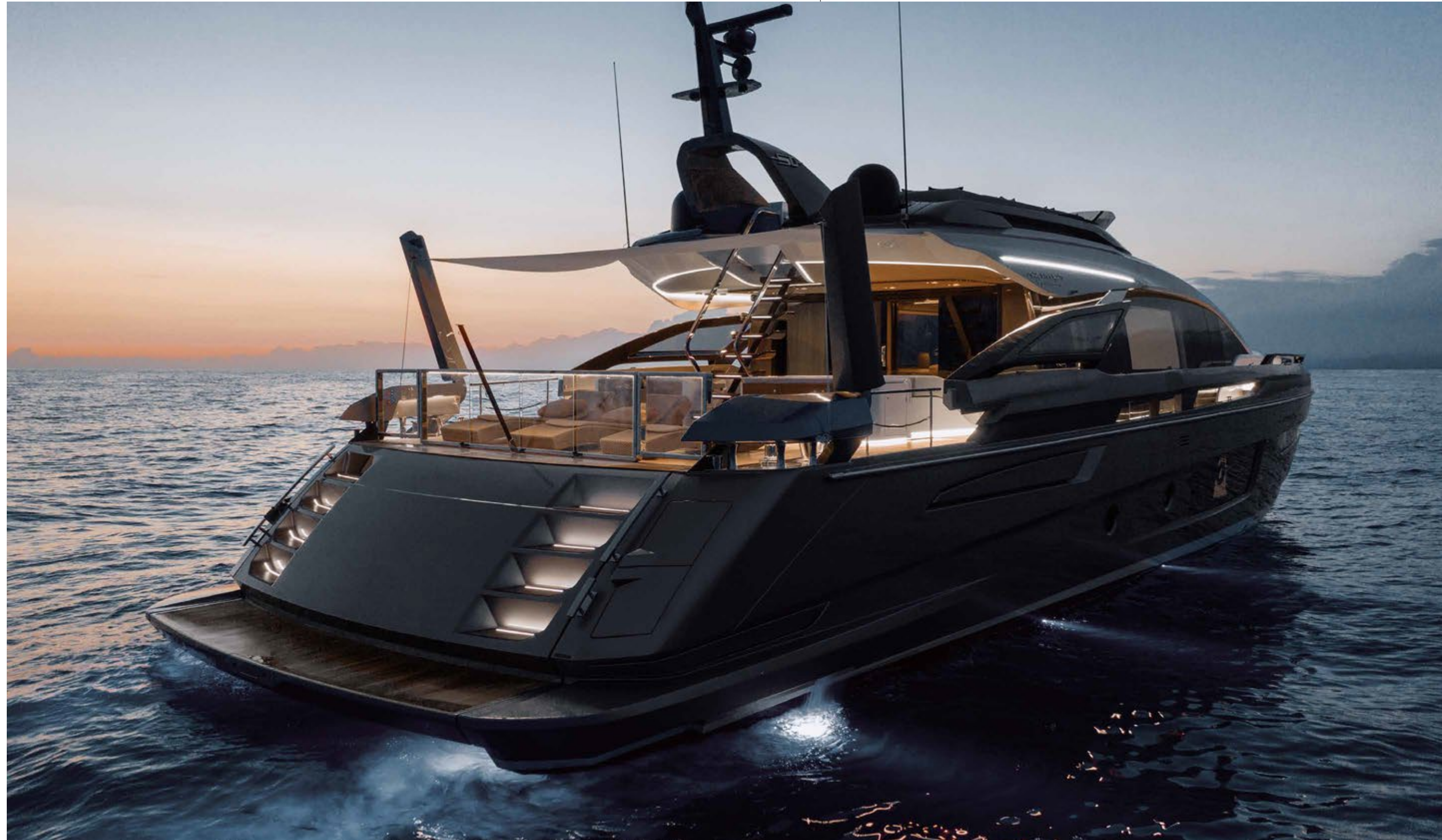
[ Light design elements combine the functional and the aesthetic LED lights to spotlight the steps to the stern swim platform and the vertebral stairway to the flybridge. When activated, they light up in a choreographed sequence, making a strong first impression. ]
